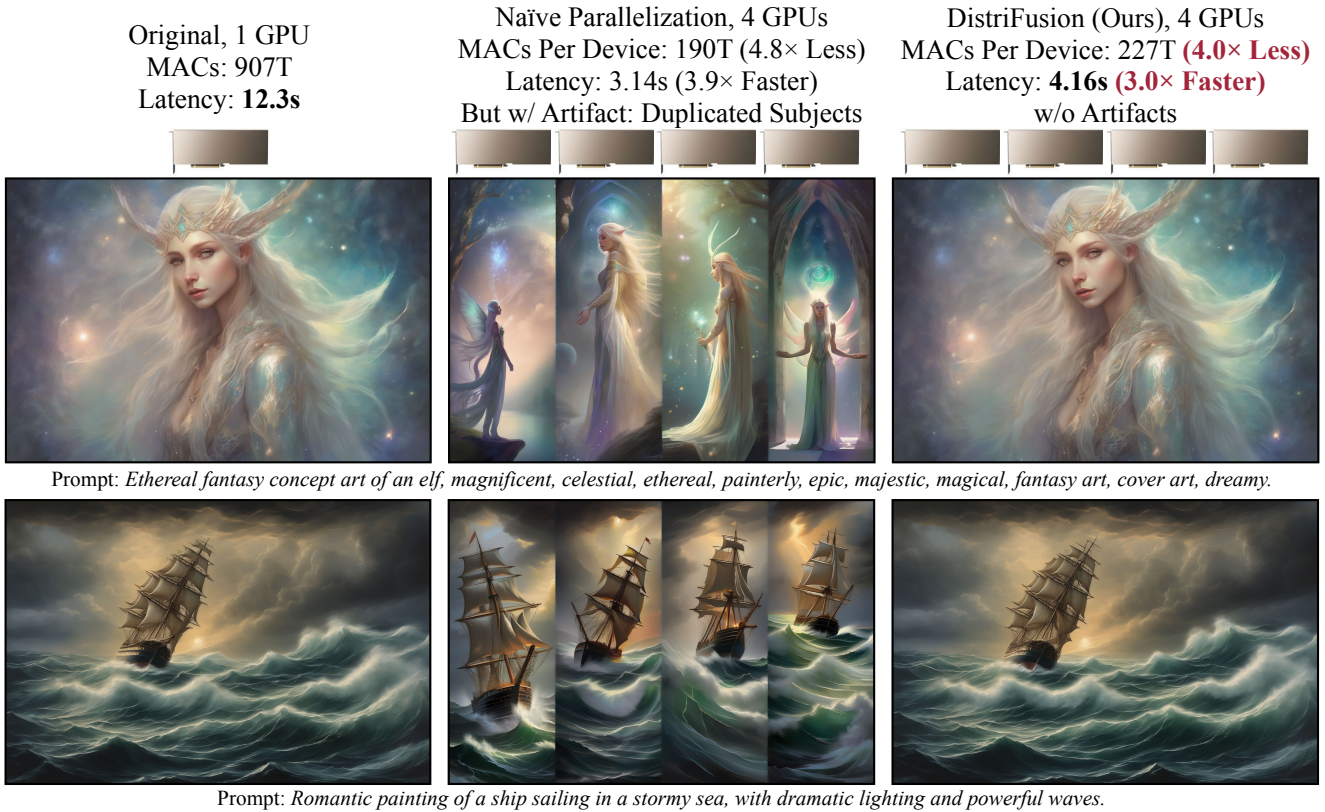
Figure 1. We introduce DistriFusion, a training-free algorithm to harness multiple GPUs to accelerate diffusion model inference without sacrificing image quality. Naïve Patch (Figure 2(b)) suffers from the fragmentation issue due to the lack of patch interaction. Our DistriFusion removes artifacts and avoids the communication overhead by reusing the features from the previous steps. Setting: SDXL with 50-step Euler sampler, 1280 × 1920 resolution. Latency is measured on A100s.
