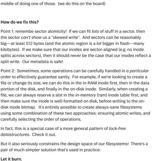
Just write a tool (usually a version of fsck) that goes through the filesystem and tries to make the internal structures sane, by restoring their data invariants. By combining an fsck-recovery with the idea of being careful about write-order, you can represent a much bigger class of filesystem designs while maintaining
