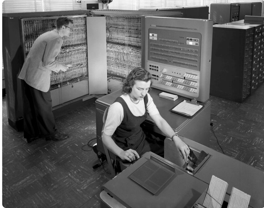
Figure 1: IBM type 704 data processing machine used for making computations for aeronautical research.
