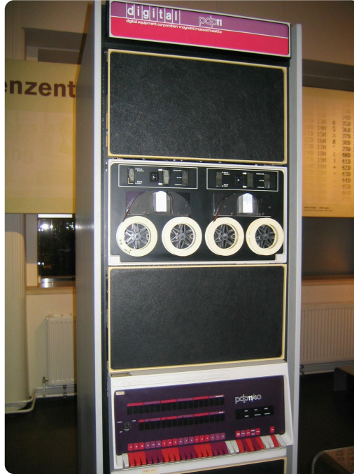
Figure 2: PDP-11, an early “minicomputers”. $1M (in 2025 $s), 10MHz CPU, 100s KB of memory.
