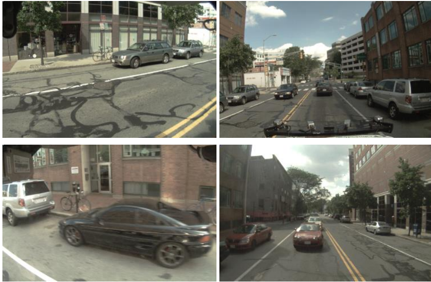
Figure 5: A scene from the urban driving data set. Starting with the image in the top left and going clockwise, they are captured with left-, forward-, right-, and rear-facing cameras mounted on the vehicle.
