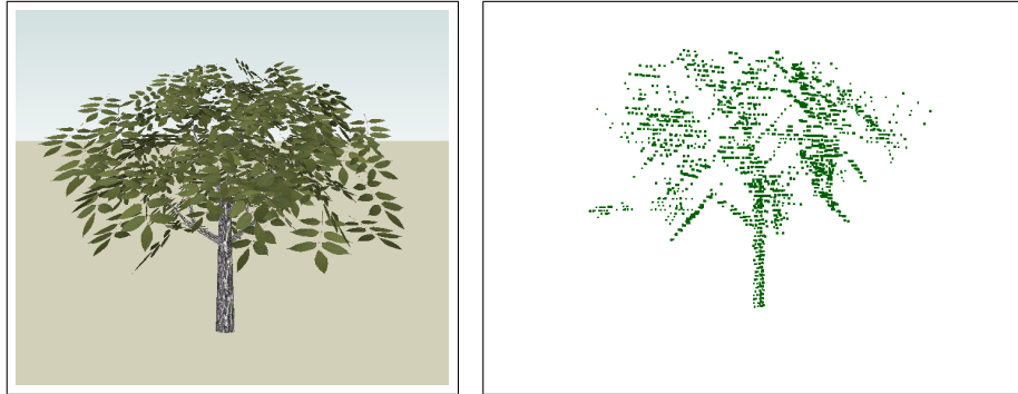
Figure 4: (left) Tree model from the 3D Warehouse and (right) point cloud extracted via ray casting.
