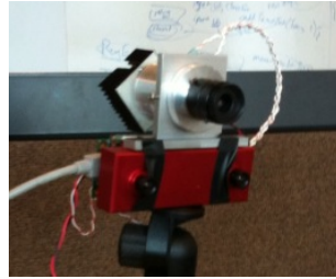
Figure 11: Stereo camera and textured light projector system.
