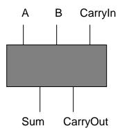
A circuit to compute a single column of an addition is called a 1-bit adder.
