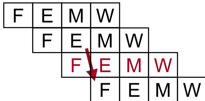
Programmer should try to insert independent instructions in branch delay slots
