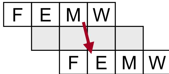
Load delay slots are inserted automatically
