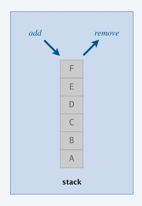
Stack. Remove the item most recently added. ← LIFO = "last in first out"
