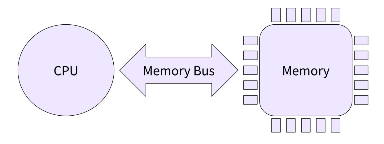
CPU connected directly to memory
