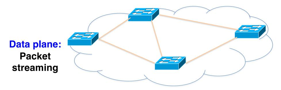
Forward, filter, buffer, mark, rate-limit, and measure packets
