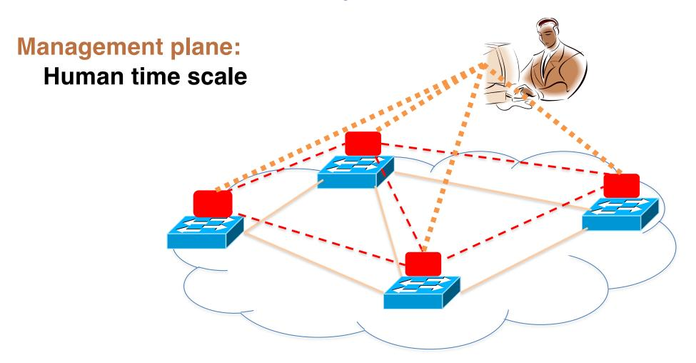
Collect measurements and configure the equipment
