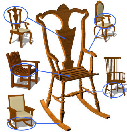
Figure 3: Modeling-by-example proposed a novel model synthesis possibility by directly composing parts retrieved from a database of 3D shapes [Funkhouser et al. 2004]. As 3D model repositories continue to grow, such a design possibility has increasingly gained research focus.
