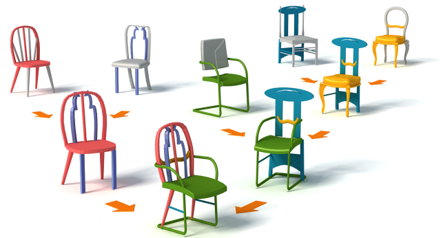
Figure 25: Evolution paths leading to the generation of a chair (bottom) with a new structure [Xu et al. 2012a]. Note that new topologies can be generated by the crossover operator. The ancestors of the final chair belong to sets of shapes that are evolved together, i.e., a set evolution.
