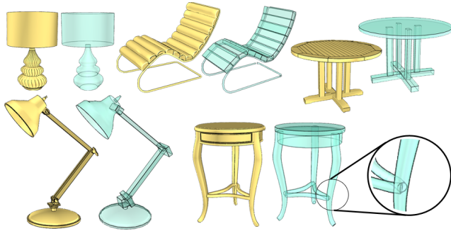
Figure 18: Controllers (shown in cyan), either a cuboid or a generalized cylinder [Zheng et al. 2011], serve as high-level deformation handles for structure-aware deformation of man-made shapes [Xu et al. 2011]. The numbers indicate the number of controllers needed, showing that a small number of controllers usually suffice for the modeling tasks.
