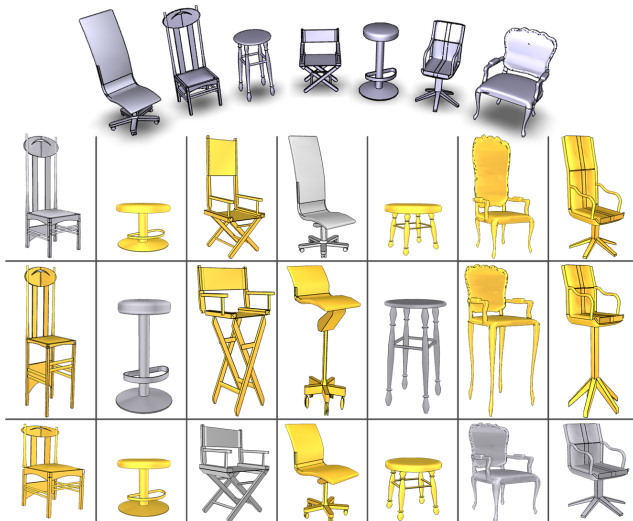
Figure 10: Style-content separation [Xu et al. 2010] by anisotropic part scales facilitates part correspondence among a diverse set of chairs (top). The separation is shown by the table with rows representing identified styles. The correspondences allow automatic synthesis of novel shapes (shaded in gold) from the example set via style transfer.
