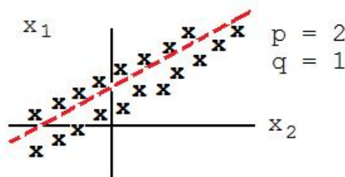
Figure 1: A plot of x 's in 2D ( \mathbb{R}^p ) space and an example 1D ( \mathbb{R}^q ) space (dashed line) to which the data can be projected.
