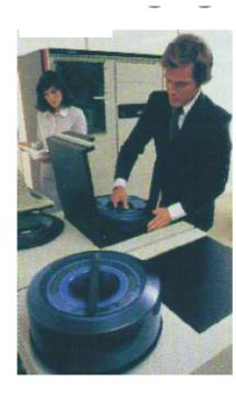
First Disk: IBM 305 RAMAC (1956) 5MB capacity 50 disks, each 24"
